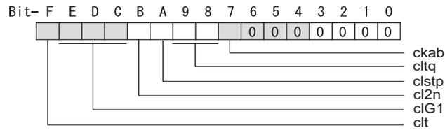
**bit F : clt Inertia ratio display**
