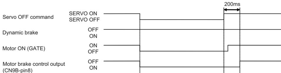
Motor brake control sequences when a servo OFF command is output
