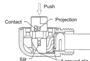
Adjust the projection of receptacle housing to the slit of the receptacle case and push in until it is fixed to the case.
