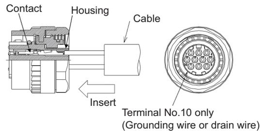
(Note) Before inserting the contact, check that the clamp nut, cable clamp, bushing and back shell is inserted.
