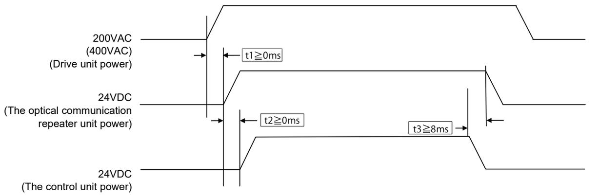
t1: Time lag between the power-ON of the drive unit and the optical communication repeater unit
