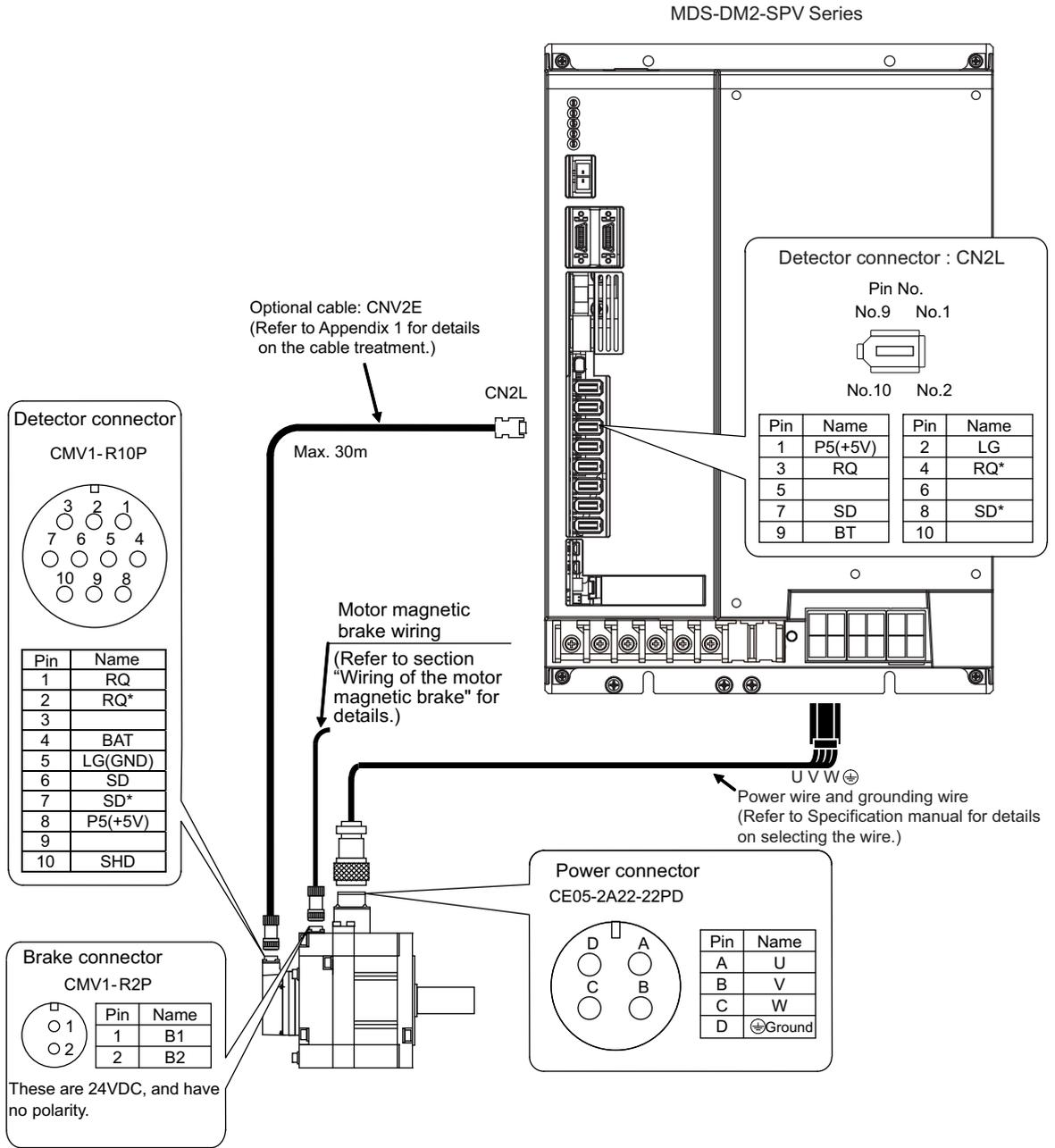
2.5.2 Connection of the full-closed loop system
