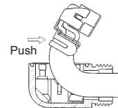
When the ground clip interferes with receptacle case at the position in the right figure and cause difficulty in continuing to draw in, push the ground clip to distort and drawing become easy.
