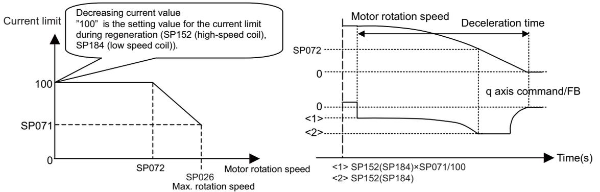
**【#13071】 SP071 DIQM Variable current limit during deceleration, lower limit value**
