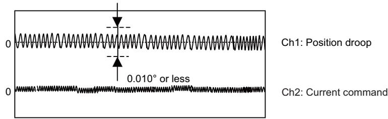
\* Waveform when executing cutting feed with G01 F20 (Reference)
