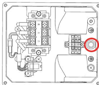
Section where the cooling fan lead wires are led out
