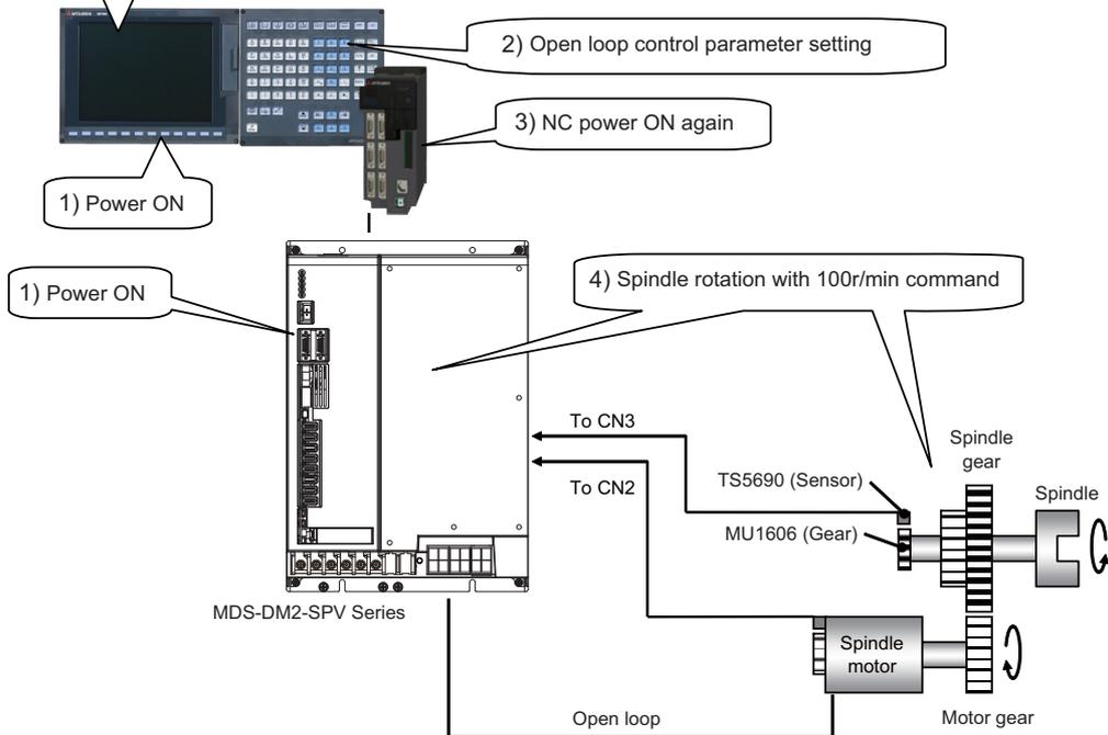
Installation diagnosis for spindle side PLG encoder
