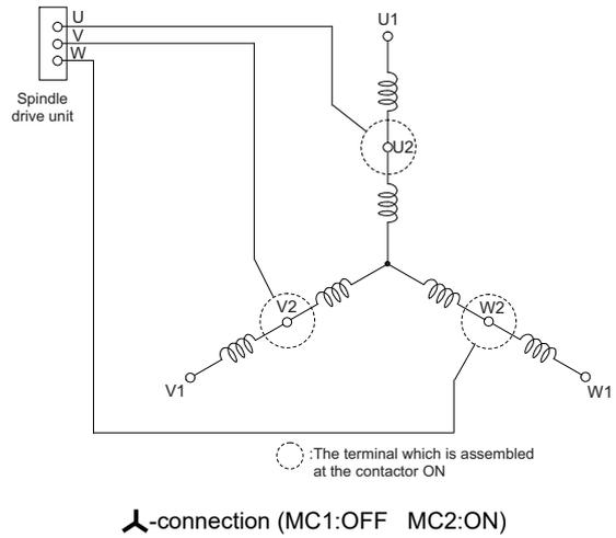
○:The terminal which is assembled at the contactor ON
