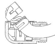
(Note) To prevent a fracture, do not use the ground clip which is bend and unbend 3 times or more.
