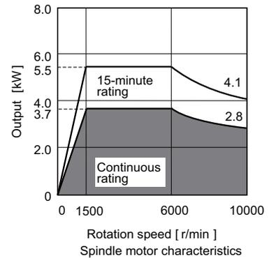
$$t_1 = \frac{1.097 \times 10^{-2} \times J_{all} \times N_1^2}{P_o} = \frac{1.097 \times 10^{-2} \times 0.0648 \times 1500^2}{6600} = 0.242 \text{ [s]}$$
