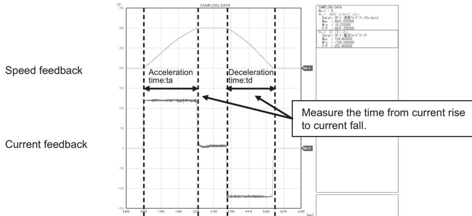
Acceleration/deceleration characteristics of spindle motor
