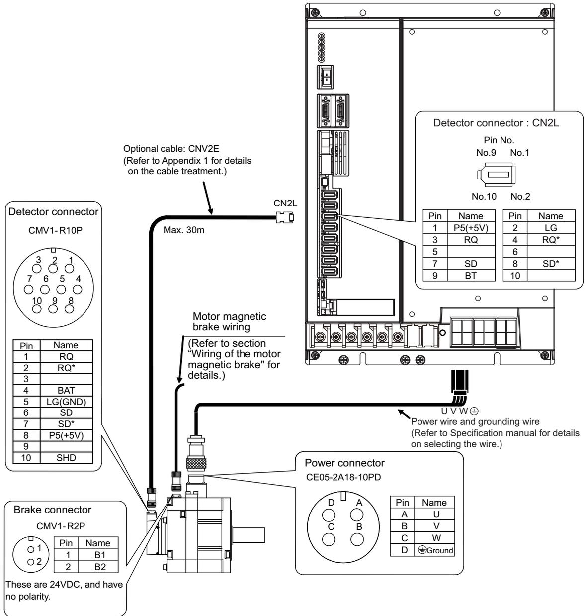
(2) Connecting the HF204(B) / HF354(B) / HF303 / HF453 / HF302
