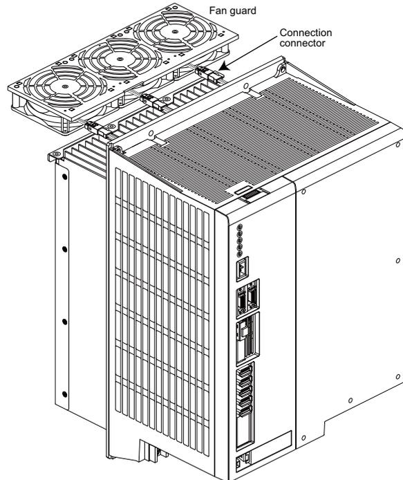
[3] Disconnect the fan connection connector.
