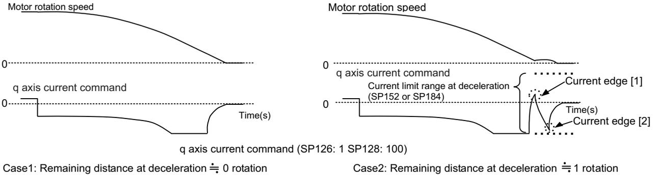
**【#13016】 SP016 DDT Phase alignment deceleration rate**
