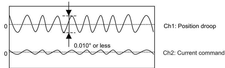
[2] When satisfactory accuracy is not secured, increase SP008 (VGN2) by 10 increments and adjust so that the accuracy level meets the standard. Note that the maximum setting value is 150 x [inertia ratio].
