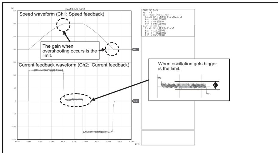
(Example)As the closest value should be selected from the standard setting range shown below, set 47 to SP001 when the limit gain is 55.
