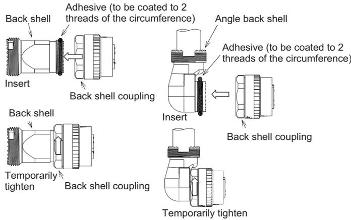
\* When tightening temporarily, match the concavity and convexity of the plug shell with those of the back shell. (You can confirm the correct connection of concavity and convexity waving lightly back shell just before inserting to BS coupling.)
