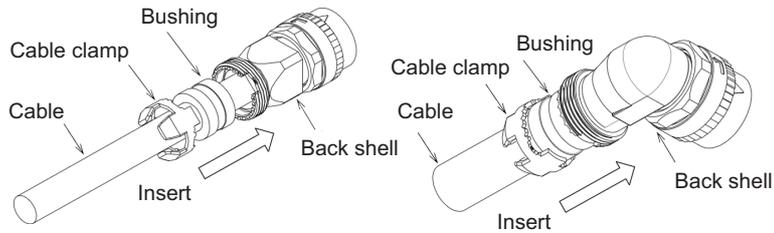
(Note) After the Bushing insert, confirm that cable position should be inside of Bushing.
