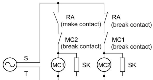
**Coil changeover relay control circuit**
