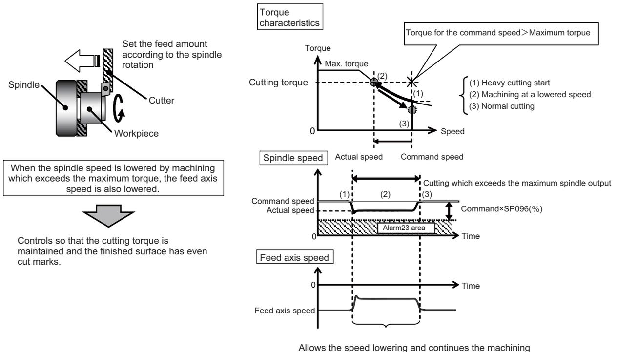
When the spindle speed is lowered by machining which exceeds the maximum torque, the feed axis speed is also lowered.
