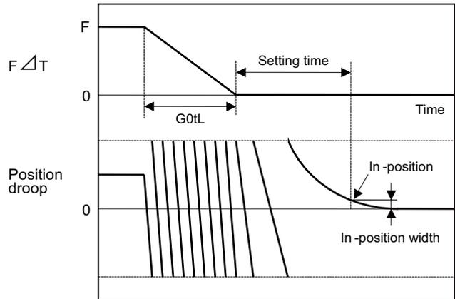
$$\text{Settling time ( ms )} = \frac{10^3}{\text{PGN1}} \cdot \ln \left[ \frac{F \times 10^6}{60 \times \text{G0tL} \times \text{PGN1}^2} \times \left[ 1 - \exp \left[ - \frac{\text{PGN1} \times \text{G0tL}}{10^3} \right] \right] \right] \text{INP}$$
