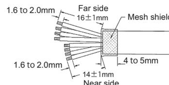
(Note) Even when the dimensions above is applied, product performance problem can occur depending on the wires which is used.
