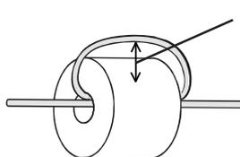
The clearance between the ferrite core and cable must be as narrow as possible when winding a cable.
