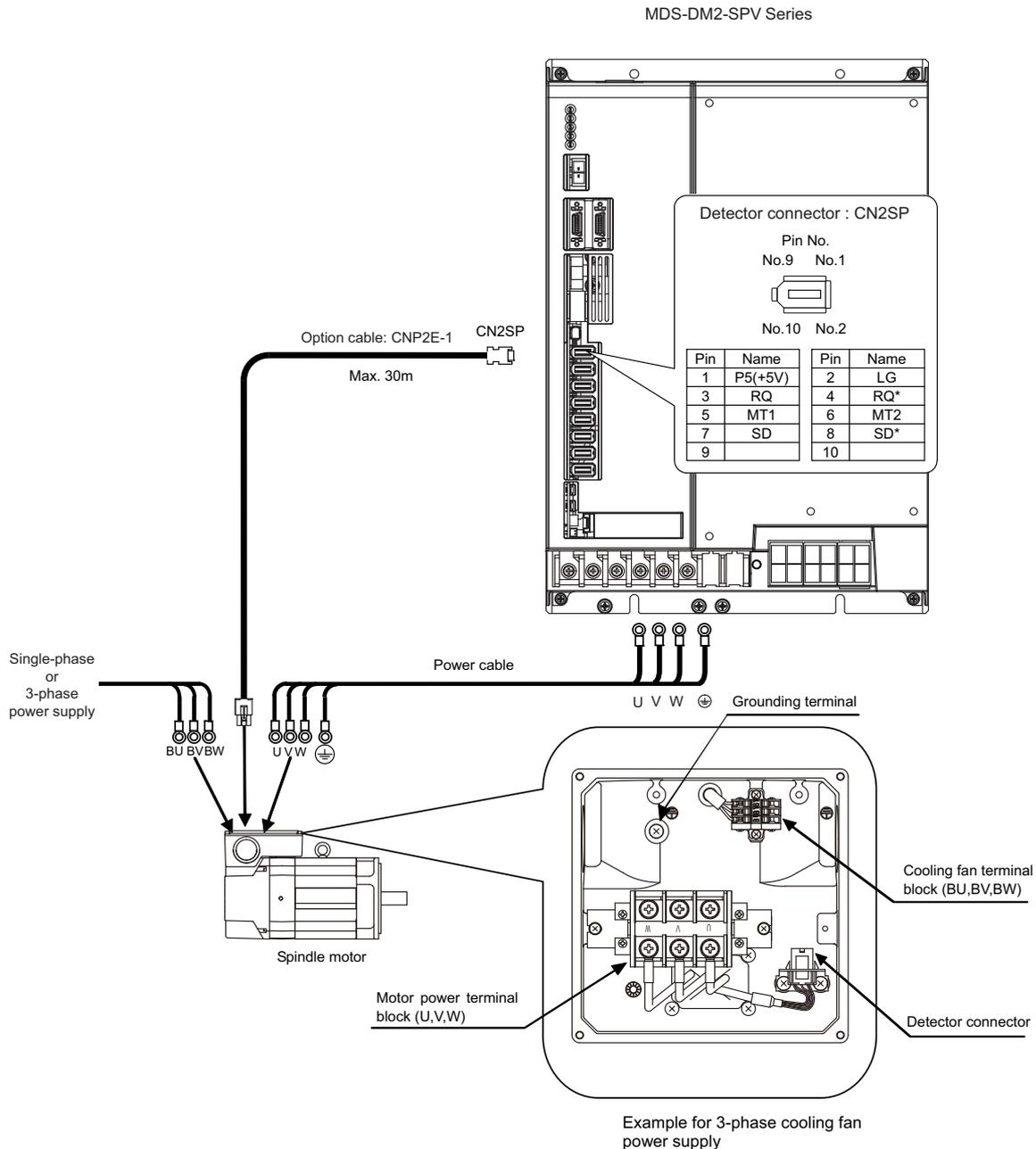
**(Note)** Either a single-phase or 3-phase power supply is used for the cooling fan. Refer to the Spindle Motor Specifications for details.
