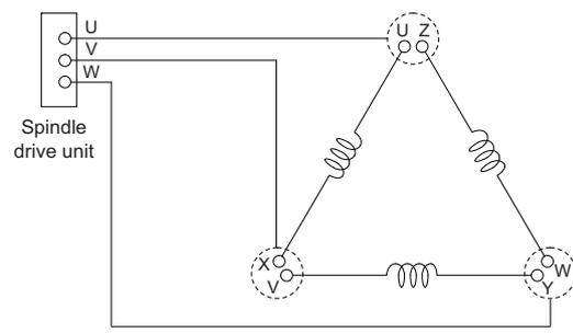
$\Delta$ connection (MC1:OFF MC2:ON)
