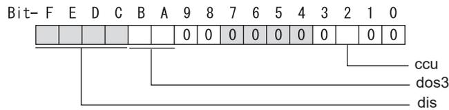
**bit F-C : dis Digital signal input selection**
