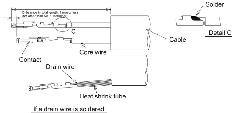
**(5) Inserting the contact**
