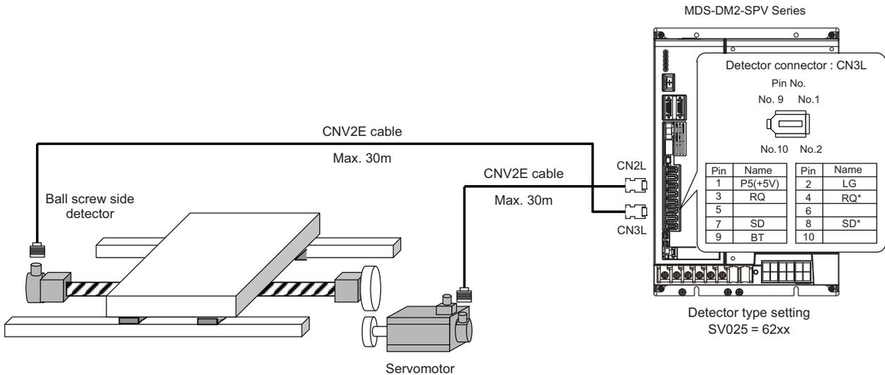
(2) Connecting the linear scale (For Mitsubishi serial signal output)
