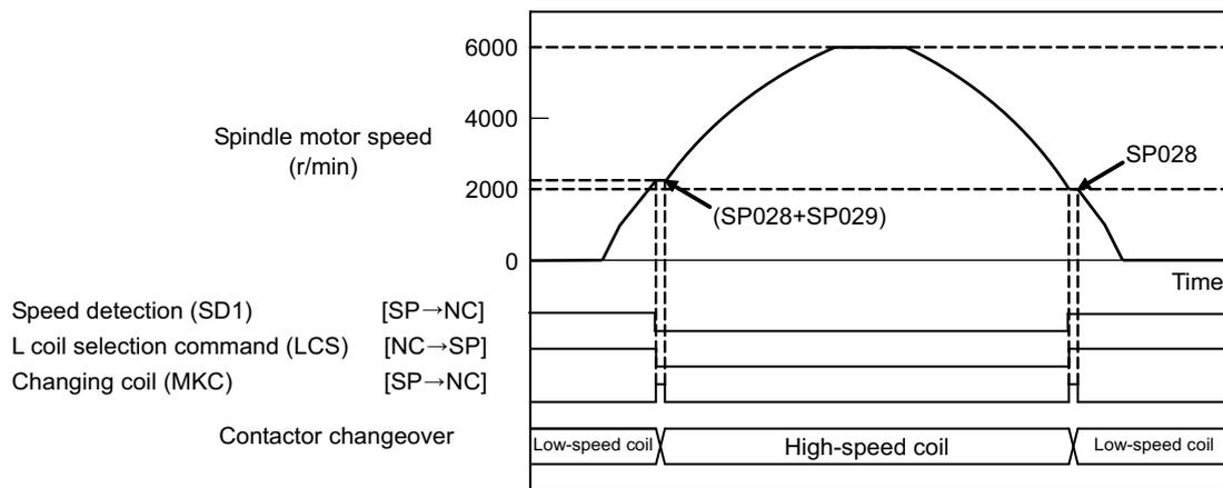
**Spindle motor coil changeover control**
