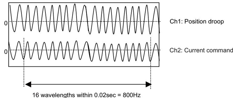
Set 800 to SP038 and XXX0 to SP034. Measure position droop and current command at this time, and adjust notch filter's frequency and depth so that the position droop is within standard range.
