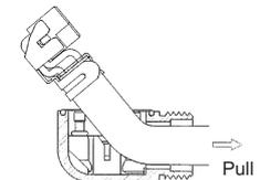
Work will become easy when the crimping part of the ground clip is pushed and the cable is bent as shown in the right figure.
