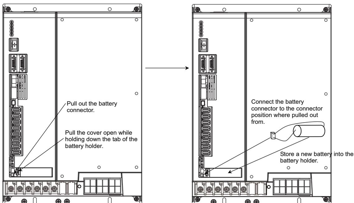
**< Replacement procedure for the battery unit MDS-BTBOX-36 >****Possible backup period**
