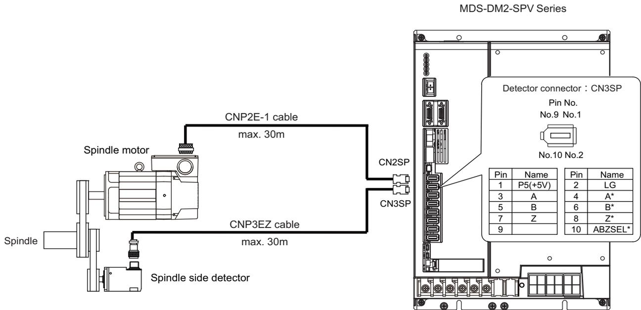
(Note) Confirm that the gear ratio (pulley ratio) of the spindle end to the encoder is 1:1. Use a timing belt for connecting.
