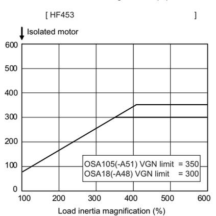
**(2) Setting the speed loop lead compensation**
