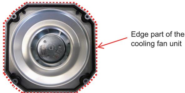
(Note 3) Do not grip the cooling fan lead wire (including the protection tube) when carrying the cooling fan unit. Carrying with gripping them may result in damages of the fan unit.
