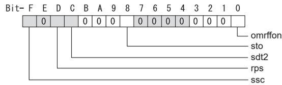
**bit F : ssc SLS (Safely Limited Speed) function**
