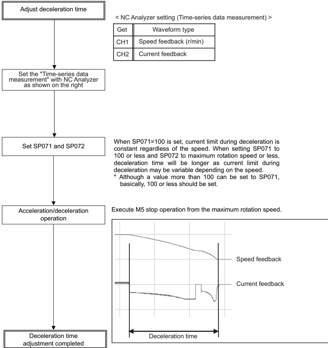
Relation between SP071 (variable current limit during deceleration, lower limit value) and SP072 (variable current limit during deceleration, break point speed)
