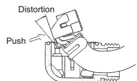
Turn the form of the ground clip back to normal and position it for the receptacle case as shown in the right figure.
