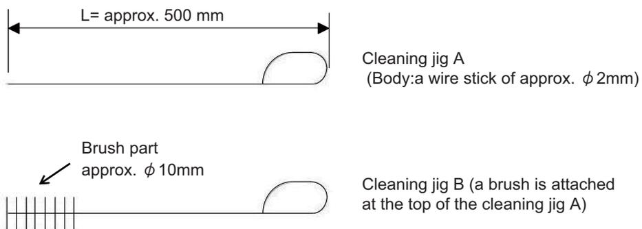
[3-2] Use the cleaning jigs to clean the air ducts of the spindle motor frame.
