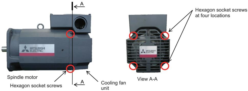
(Note 1) Some spindle motors have the fixing screws (hexagon socket screws) for the cooling fan unit at two locations.
