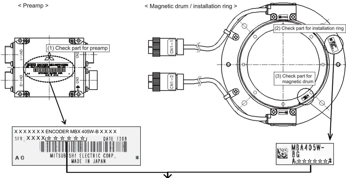
Make sure that the serial Nos. (☆ 6 digits) of the nameplate stickers attached on the above three parts are the same.
