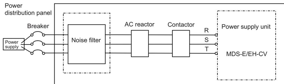
(Note) The noise filter must be prepared by the user.
