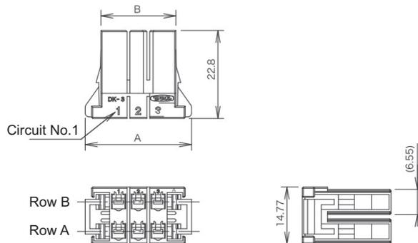
Connector for CN23 (Connector for contactor control output)
