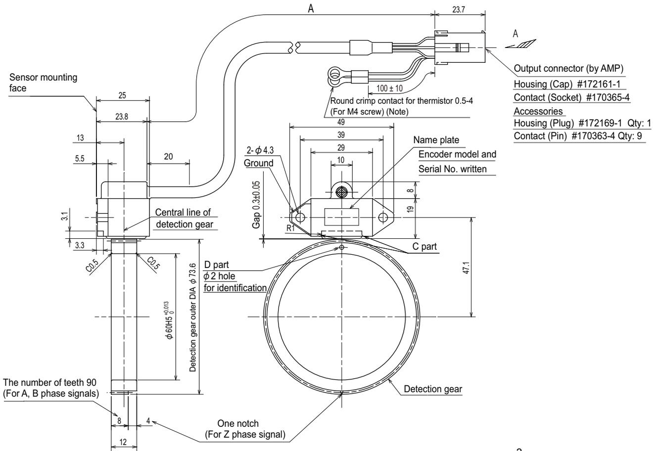
(Note) The thermistor contact is not used when the encoder is used as a spindle side encoder. Insulate the terminal.
