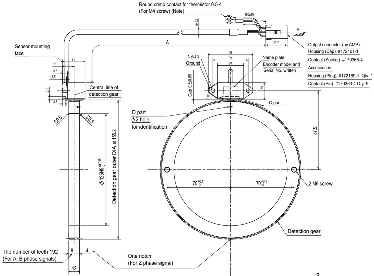
(Note) The thermistor contact is not used when the encoder is used as a spindle side encoder. Insulate the terminal.
