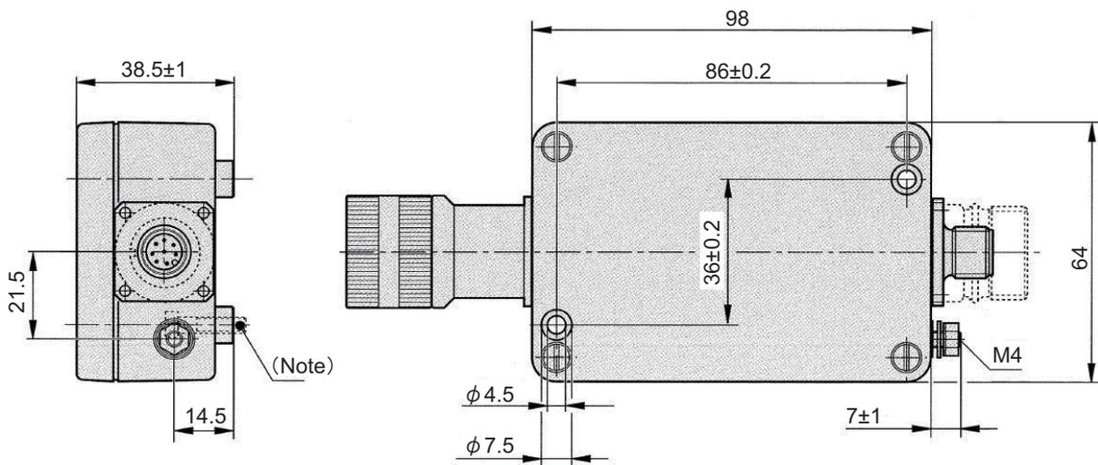
(Note) Two fixing screws (M4×16 DIN 912/ISO 4762)
