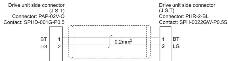
(Note) Shield processing of battery cable is unnecessary.
