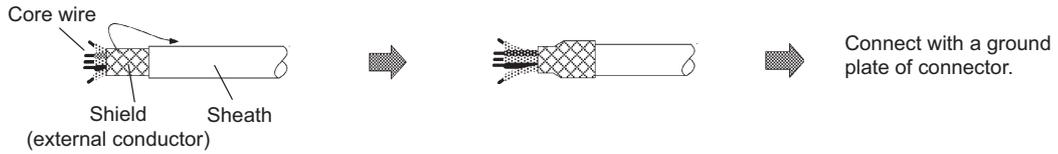
(Note) Shield processing of battery cable is unnecessary.
