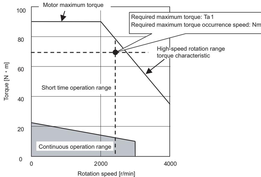
**Motor torque characteristics**
