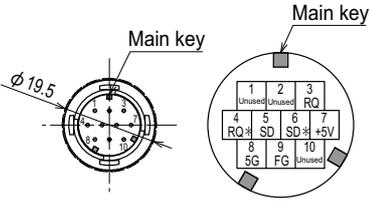
Seen from Arrow A Pin layout of output connector
