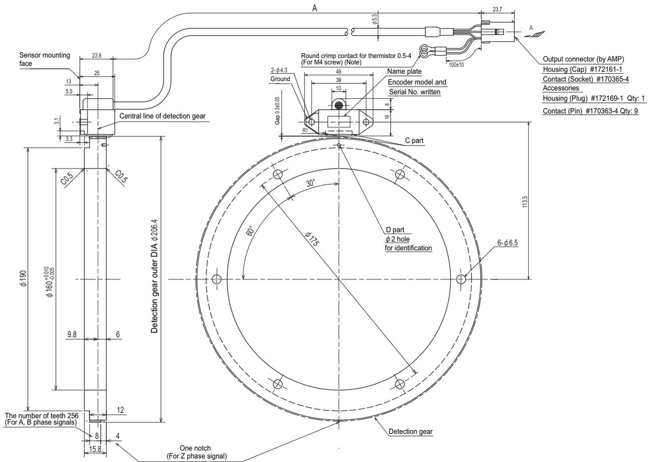
(Note) The thermistor contact is not used when the encoder is used as a spindle side encoder. Insulate the terminal.
