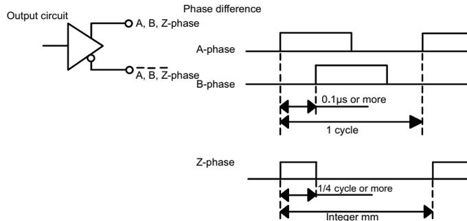
(Note 1) For a scale having multiple Z phases, select the neighboring Z phases whose distance is an integer multiple or 1/integer of the ball screw pitch.
