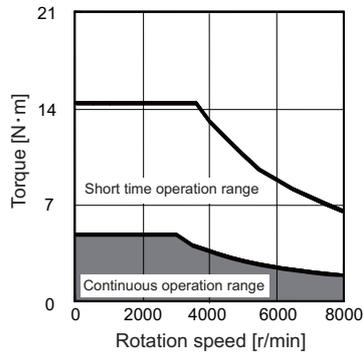
(Note) The above graphs show the data when applied the input voltage of 380VAC. When the input voltage is 380VAC or less, the short time operation range is limited.
