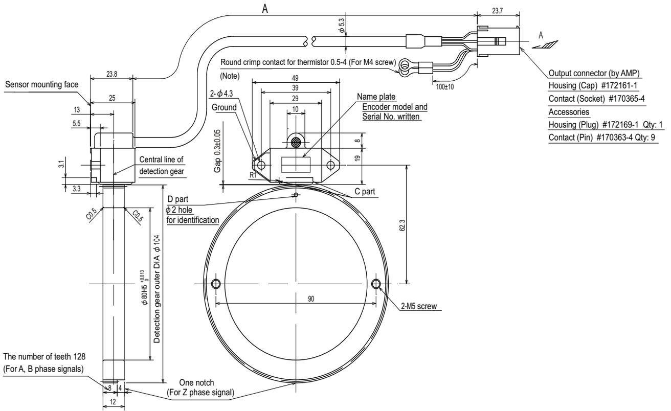
(Note) The thermistor contact is not used when the encoder is used as a spindle side encoder. Insulate the terminal.
