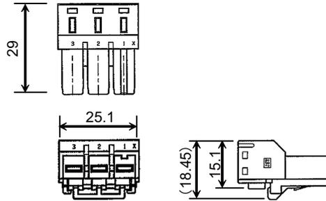
Connector for CN24 (Connector for external emergency stop)
