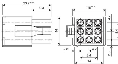
Spindle side encoder connector (for OSE-1024)
