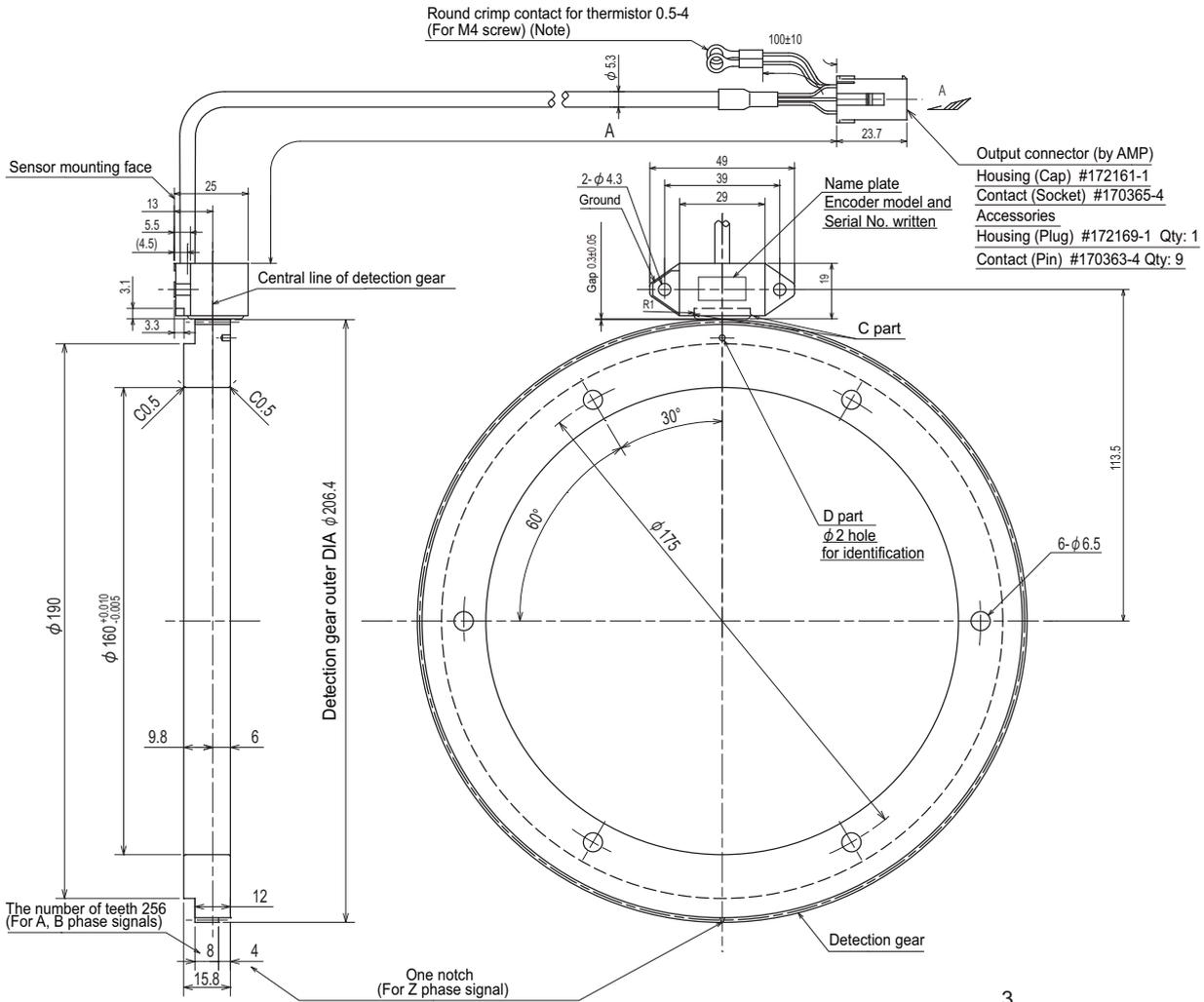
(Note) The thermistor contact is not used when the encoder is used as a spindle side encoder. Insulate the terminal.
