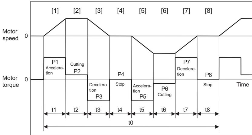
Output during acceleration/deceleration (kW)
