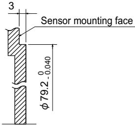
Encoder mounting face of machine side
