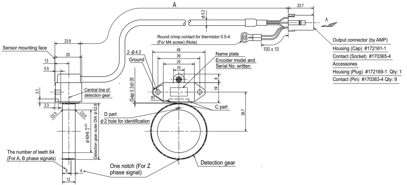
(Note) The thermistor contact is not used when the encoder is used as a spindle side encoder. Insulate the terminal.
