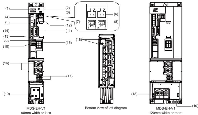
The connector and terminal block layout may differ according to the unit being used. Refer to each unit outline drawing for details.
