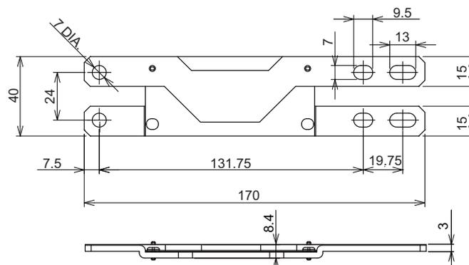
(Note) E-BAR-A0606 is a set of two DC connection bars.
