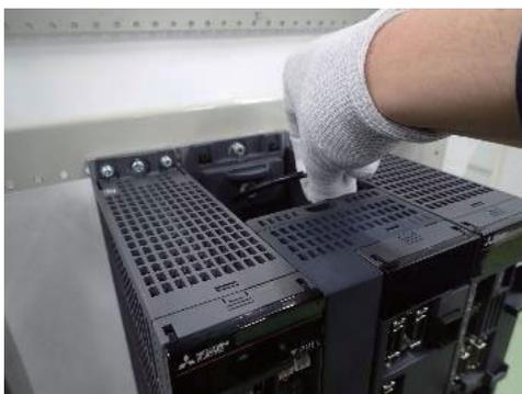
Set the connector to the start position. Slide the connector down the slide and insert it. Pay attention to which side the locking part of the connector is facing (the locking part should face the inner side of the unit).
